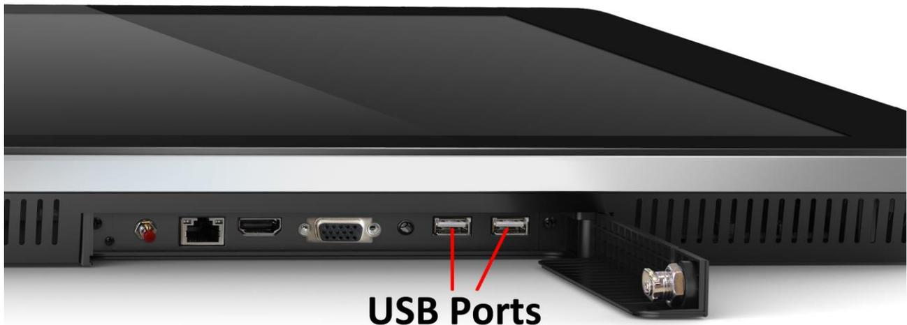
Figure 1 Position of screen inputs
