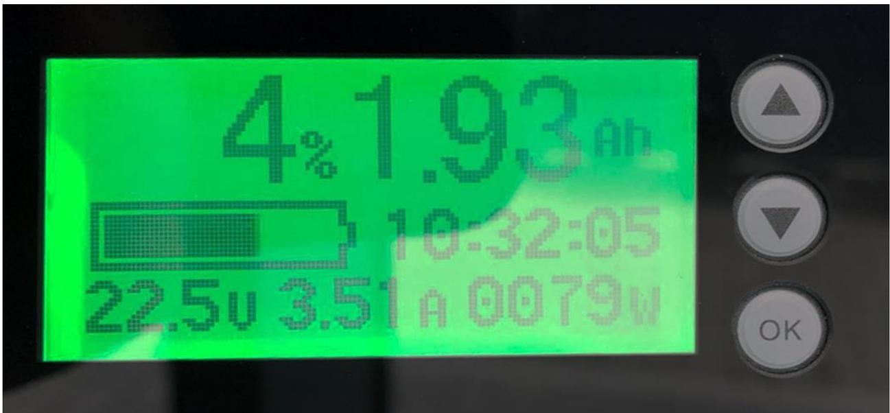
Figure 8. Charge Level Indicator
