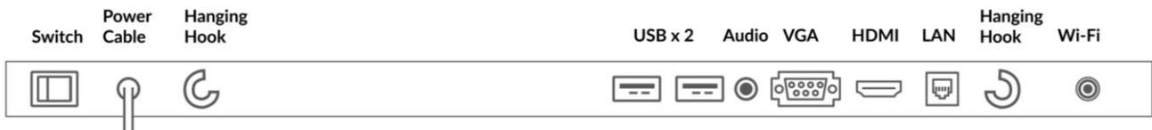
Figure 9 Top view of display
