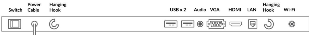
**Figure 8** Top view of display
