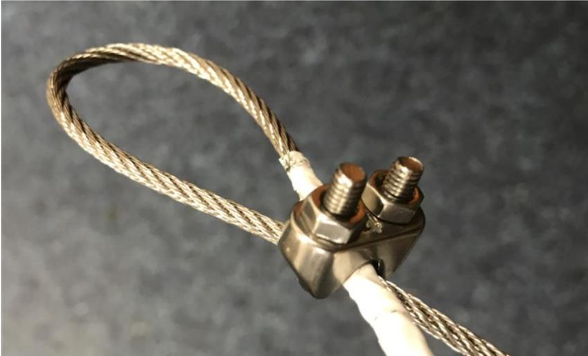
6. Cut off any excess wire rope.
